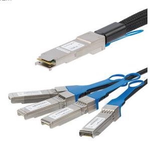
The QSFP4SFPPC2M is an MSA Compliant QSFP+ direct-attach Twinax breakout cable. It is designed, programmed and tested to bridge 40G network equipment with 10G compatible servers or routers. This passive Twin axial cable connects a single QSFP+ port to four 10G SFP+ ports and is fully hot-pluggable making upgrades and replacements seamless by minimizing network disruptions.
